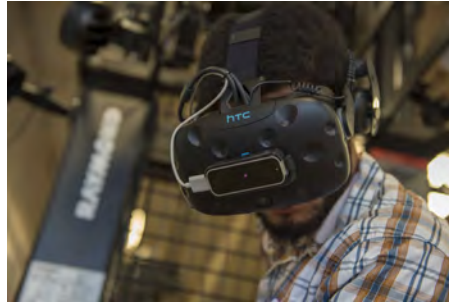
A worker using Raymond Corporation's virtual reality forklift simulator
